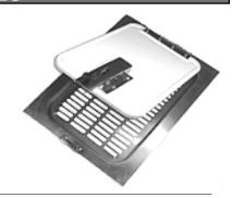
**Skylights** are molded in one piece from shatter-proof translucent fiberglass reinforced plastic. Supplied complete with self-sealing rubber grommet. For installation into 12" or 16<sup>3</sup>/<sub>16</sub>" diameter holes. Easy snap-in installation with grommet cord.
